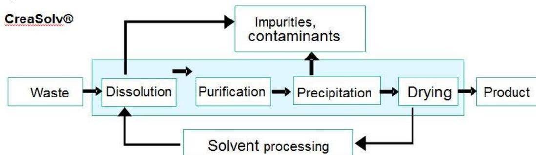
Picture 2 CreaSolv process flow diagram
