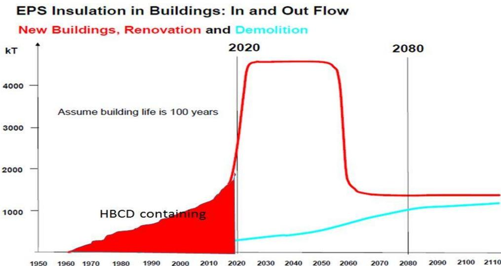
Picture 1 PS foam used incl HBCDD plus the upcoming release of B&C insulation foam during demolition
